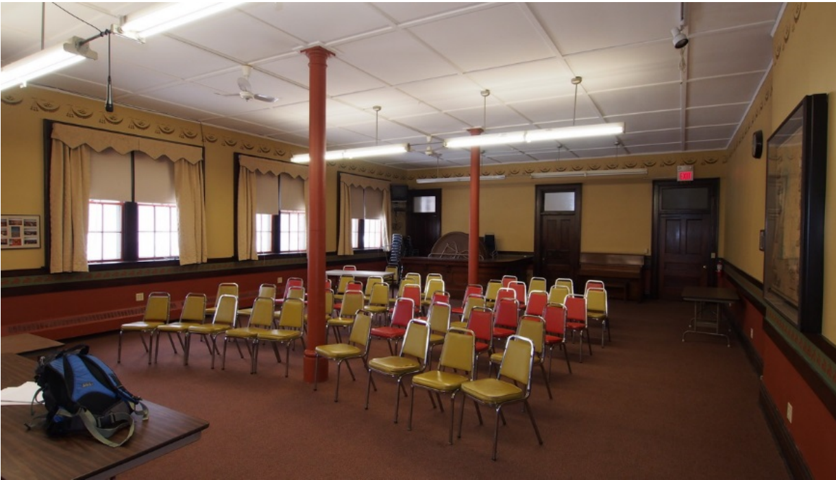
Banquet hall showing carpeted floor, lowered panel ceiling, steel bearing columns, plaster wall finish and chairrail.
